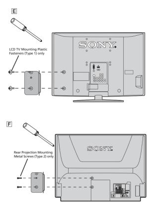
**2** Take the bracket and match the holes on the bracket to the screw holes on the back of your TV.
